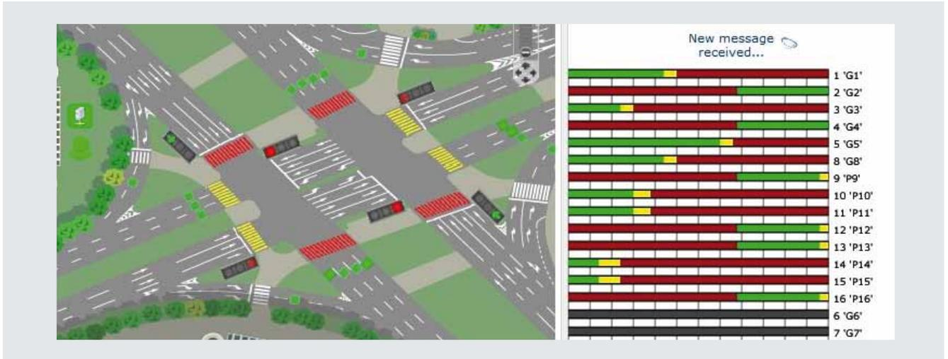
■ The operator can visualise any system at network scale or zoom in to understand the detailed conditions. It is possible to check the location of buses, the fluidity of traffic, the messages being displayed on overhead panels, the occupancy of car parks, whether the street lighting is on.....
